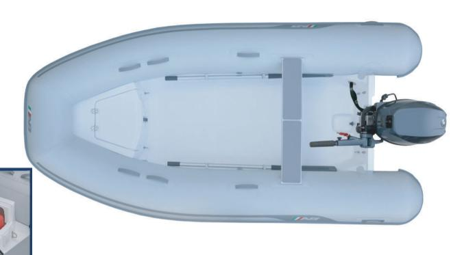
ے S **Overal Length** : 12′/ 3.66m Number of Chambers : 3 + 1Shaft Length Option 1: 15"/38.1cm Shaft Length Option 2:20"/50.8cm **Person Capacity Overal Beam** : 6′/ 1.82m : 6 Inside Length Weight : 202lb / 92kg RDC Design Category: C : 8'9"/ 2.67m Inside Beam Recommended HP : 2'9"/ 0.84m : 20hp / 14.9kw **Tube Diameter** : 18"/ 0.46m Maximum HP : 30hp / 22.4kw
