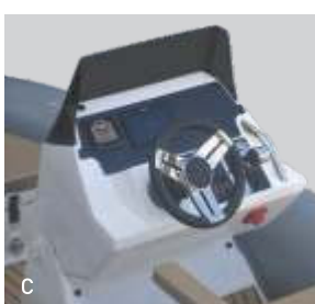
PICTURE A SINGLE LEVER THROTTLE WITH ELECTRONIC CONTROL
