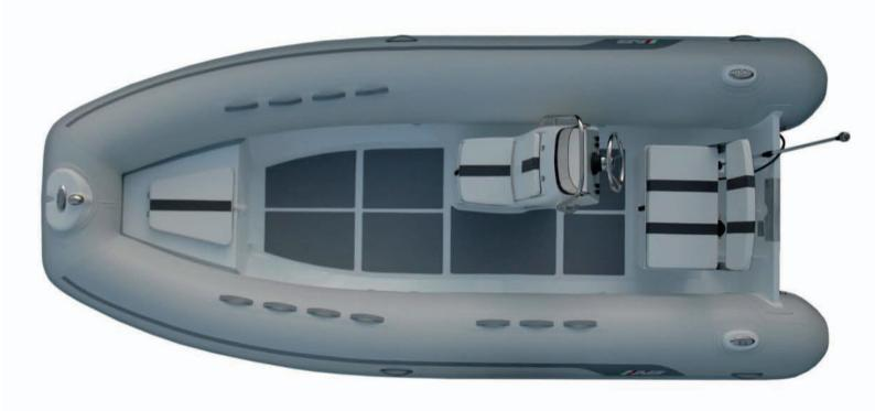
Overal Length : 16'/ 4.88m Number of Chambers : 5 Shaft Length : 20" / 50.8cm **Person Capacity** : 10 RDC Design Category : C **Overal Beam** : 7′/ 2.14m
