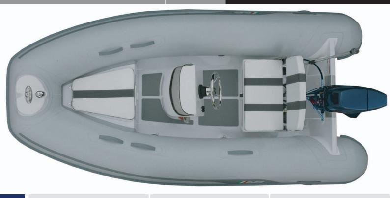
Overal Length : 9'6"/ 2.90m Number of Chambers : 3 Shaft Length : 20" / 50.8cm **Person Capacity** RDC Design Category : C **Overal Beam** : 5 : 5′6″/ 1.68m : 6′11″/2.11m Inside Length Weight : 249lb / 113kg
