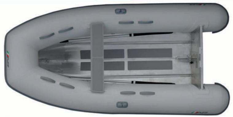
**Overal Length** Shaft Length : 10'/ 3.05m Number of Chambers : 3 : 15" / 38.1cm Overal Beam **Person Capacity** : 5'6"/ 1.68m RDC Design Category : C Inside Length : 7'2"/ 2.18m Weight : 95lb / 43kg Inside Beam : 2'8"/ 0.81m Recommended HP : 8hp / 6.0kw Maximum HP **Tube Diameter** : 17"/ 0.43m : 9.9hp / 7.4kw
