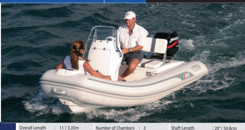
Overall Length : 11′/3.35m **Number of Chambers Overall Beam Person Capacity** : 5 : 5'8"/1.73m Inside Length : 370lb / 168kg : 8'1"/ 2.47m Weight
