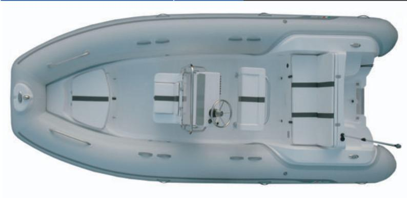
Overall Length : 19′/ 5.79m Number of Chambers : 5 Shaft Length **Person Capacity** Gas Built in Tank Overall Beam : 8'4"/2.53m : 15 : 14'11"/ 4.55m Inside Length Weight : 1252lb / 569kg Water Built in Tank Recommended HP Inside Beam : 4'4"/1.32m :115hp / 85.8kw RDC Design Category: C :150hp / 111.9kw **Tube Diameter** : 22"/ 0.56m Maximum HP
