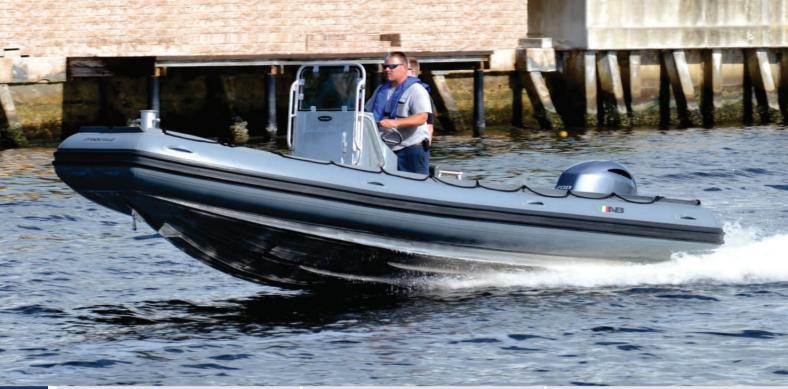
**Overal Length** : 21′/ 6.4m Number of Chambers : 6 **Overal Beam Person Capacity** : 17 : 9'1"/2.77m
