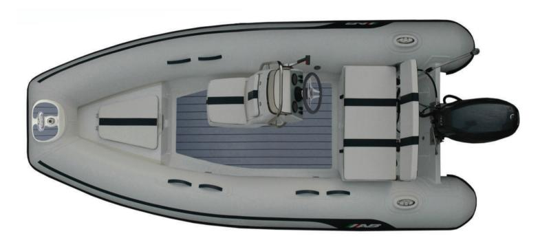
**Overal Length** : 13′/ 3.96m Number of Chambers : 3 Shaft Length : 20" / 50.8cm **Overal Beam Person Capacity** : 7 RDC Design Category : C : 6'7"/ 2.00m Inside Length : 9'10"/3.00m Weight : 372lb / 169kg Inside Beam Recommended HP : 3'3"/ 0.99m : 30hp / 22.4kw **Tube Diameter** : 18"/ 0.46m Maximum HP : 40hp / 29.8kw
