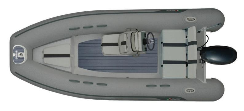
**Overal Length** : 14′/ 4.27m Number of Chambers : 4 Shaft Length : 20" / 50.8cm **Overal Beam Person Capacity** RDC Design Category : C : 6'7"/ 2.00m : 8 : 10′10″/3.30m Inside Length Weight : 392lb / 178kg Inside Beam Recommended HP : 3'3"/ 0.99m : 40hp / 29.8kw **Tube Diameter** : 19"/ 0.48m Maximum HP : 50hp / 37.3kw
