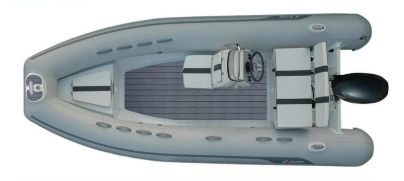
**Overal Length** : 15'/ 4.57m Number of Chambers : 5 Shaft Length : 20" / 50.8cm **Overal Beam Person Capacity** RDC Design Category : C : 6'9"/ 2.06m Inside Length : 11'8"/3.55m Weight : 467lb / 212kg Inside Beam Recommended HP : 3'4"/ 1.03m : 50hp/37.3kw **Tube Diameter** : 19"/ 0.48m Maximum HP : 60hp / 44.8kw
