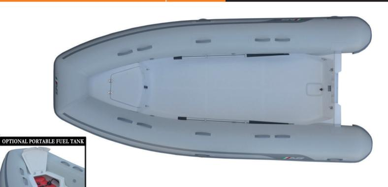
ے S **Overal Length** 14′/ 4.27m Number of Chambers : 4 + 1Shaft Length **Person Capacity** RDC Design Category : C **Overal Beam** : 6'4"/1.94m : 8 Inside Length : 10′10″/3.30m Weight : 348lb / 158kg Inside Beam Recommended HP : 3'1"/ 0.94m : 40hp / 29.8kw **Tube Diameter** : 19"/ 0.48m Maximum HP : 50hp / 37.3kw
