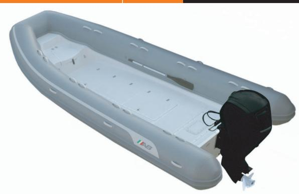
**Overal Length** : 19<sup>7</sup>/5.79m **Number of Chambers** Shaft Length : 25" / 63.5cm **Overal Beam Person Capacity** : 15 RDC Design Category : C : 8'4"/2.53m Inside Length : 15'2"/4.62m Weight : 1157lb / 526kg Inside Beam : 4'1"/ 1.25m Recommended HP : 115hp / 85.8kw Maximum HP **Tube Diameter** : 22"/ 0.56m : 150hp / 111.9kw
