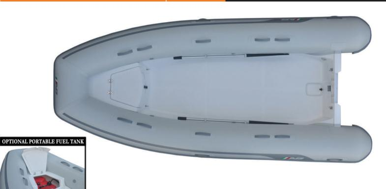
ച S Overal Length Number of Chambers : 4 + 1: 14′/4.27m Shaft Length : 20" / 50.8cm RDC Design Category : C **Overal Beam Person Capacity** : 8 6'4"/ 1.94m
