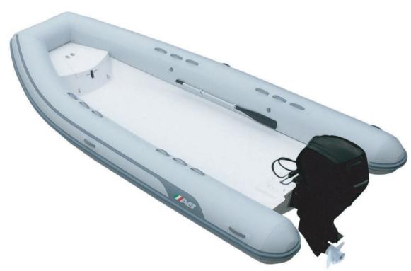
Overal Length : 17′/ 5.18m Number of Chambers : 5 Shaft Length : 20" / 50.8cm **Overal Beam Person Capacity** : 15 RDC Design Category : C : 8'1"/ 2.46m Inside Length : 13'1"/ 4.00m Weight : 772lb / 350kg Inside Beam : 4'4"/ 1.33m Recommended HP : 75hp / 56kw
