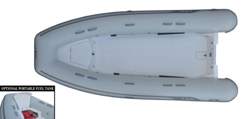
ച S Overal Length Number of Chambers : 4 + 1: 14′/4.27m Shaft Length : 20" / 50.8cm RDC Design Category : C **Overal Beam Person Capacity** : 8 6'4"/ 1.94m Inside Length : 10′10″/3.30m Weight : 348lb / 158kg
