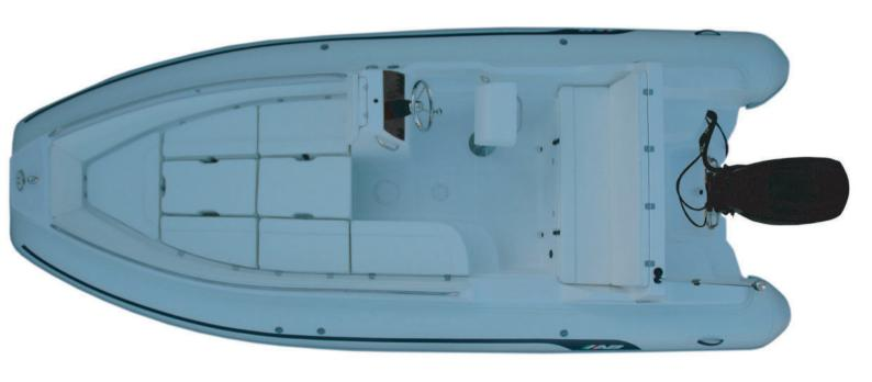
Overal Length : 19<sup>7</sup>/5.79m Shaft Length Number of Chambers: 5 : 25" / 63.5cm Gas Built in Tank **Overal Beam** : 8'4"/ 2.54m **Person Capacity** : 67 Gal / 254 L : 12 Water Built in Tank : 20 Gal / 76 L Inside Length : 15'4"/ 4.67m Weight : 1639lb / 745kg RDC Design Category : C Inside Beam Recommended HP : 4'5"/ 1.35m : 115hp / 85.8kw
