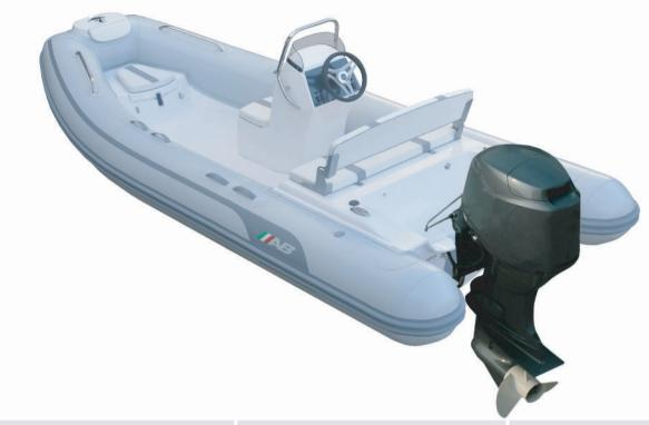
Overall Length : 15<sup>-</sup>/4.57m Number of Chambers : 5 **Overall Beam Person Capacity** : 6'6"/ 1.99m Inside Length : 11'6"/3.50m Weight : 605lb / 275kg : 60hp / 44.8kw Inside Beam Recommended HP : 3'2"/ 0.97m Maximum HP **Tube Diameter** : 19"/ 0.48m : 75hp / 56.0kw
